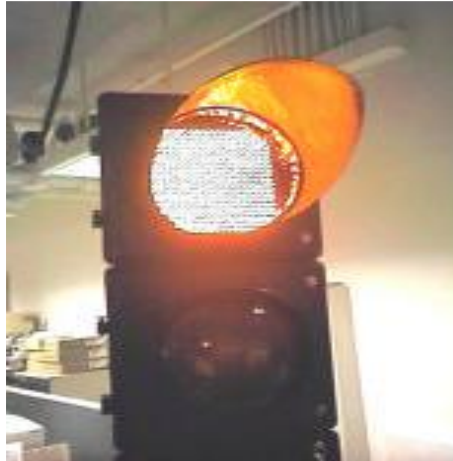
Figure-1 Photograph of a LED traffic signal
